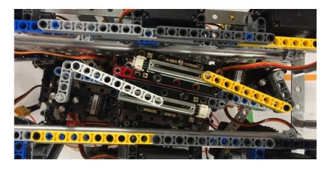
The extra pair of legs allowed the bot to hold up its 7.5 lb. weight. In addition, they allowed the bot to remain balanced and standing when a leg was raised. The legs were much more consistent with the use of servos for rotation. The feet were kept level by utilizing a shifting parallelogram in each leg. These changes fixed many of the original bot's problems but had numerous construction issues along the way.
