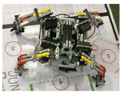
The first model used a quadruped design with a servo and motor controlling vertical movement and rotation, respectively. I originally didn't use metal in the chassis because of weight concerns, but it soon became necessary due to the entire bot folding. For traction, I utilized rubber pieces from Mindstorms. I secured the controller using a thin frame on the underside of the bot. Its gait was moving each leg up-forward-down one at a time, and then moving all back simultaneously.
