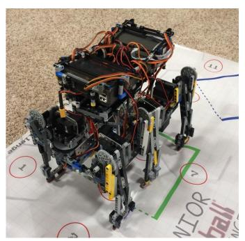
Because Botball 2019 was starting, I had to dismantle the first bot for parts. However, once the Botball season ended, I had ample parts for an improved design. The layout was much more ambitious, sporting two controllers and six legs. Two controllers allowed for double the servo and motor ports, which in turn allowed for more legs. However, this compounded the complexity of building and programming.
